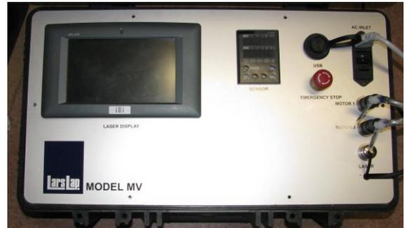
Via the USB outlet the complete measuring process can be recorded and documented into the specially developed software. The documentation shows all needed information of the valve's current condition and remaining useful life, as well as the possible need for replacement of the wedge or seat.
